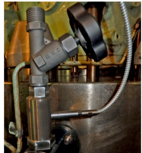
TCS-01CA sensor installed on a MAN&BW two-stroke engine
