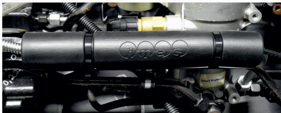
TCS-01CA sensor with protection cover installed on an engine
